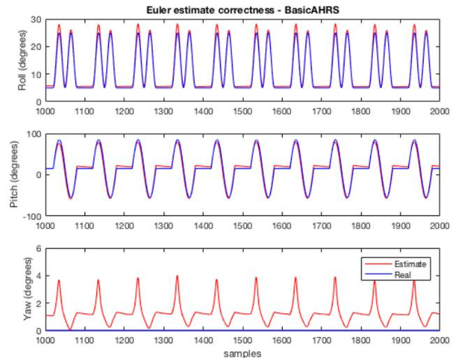
Fig. 4. Euler estimation correctness of Basic AHRS
