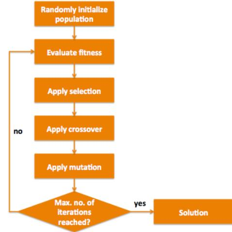
Fig. 1. Flowchart diagram of Genetic Algorithm
